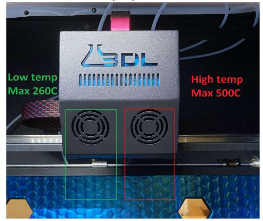
1) Hotends are installed in the following configuration out of the box
