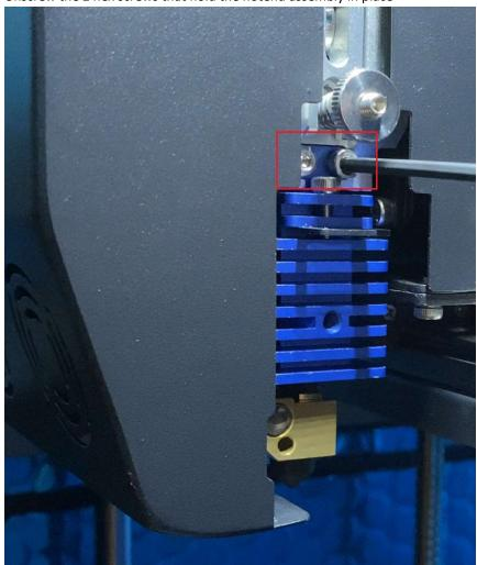
1) Unscrew the 2 hex screws that hold the hotend assembly in place
